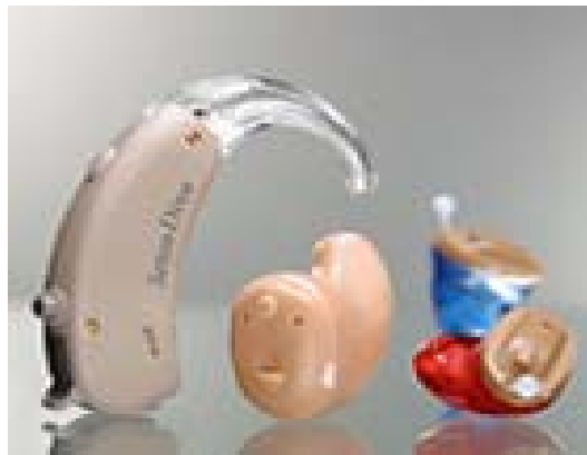
Figure (7-17): Different Styles Of hearing aids
