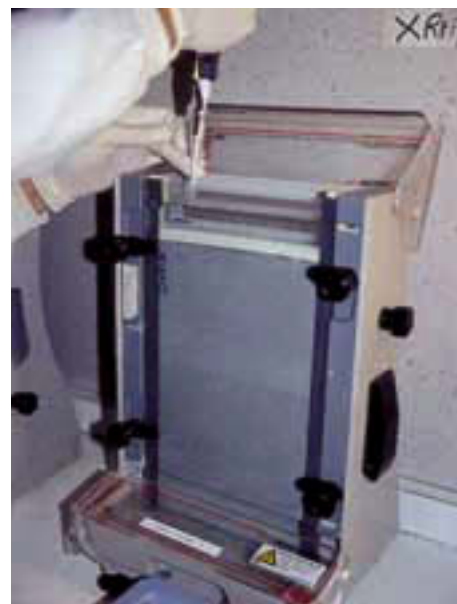
Figure 17.11 Loading PCR-amplified DNA onto an SSCP/heteroduplex gel
