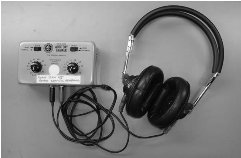
Figure 8.7 A self-contained (auditory trainer) amplification system.
