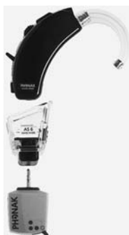
Figure 8.9 A behind-the-ear-style hearing instrument coupled with an audio “shoe” and a wireless FM receiver. (Reprinted with permission from Phonak Ear, Inc.)
